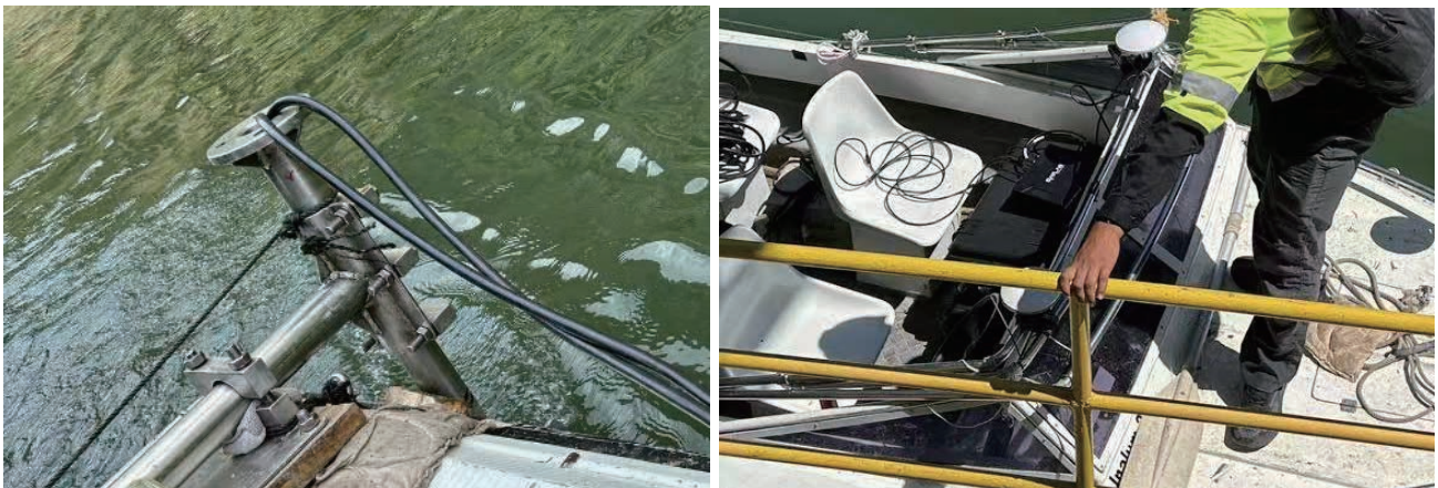
Figure 4: HydroBeam M4 Installed on Small Manned Survey Vessel
